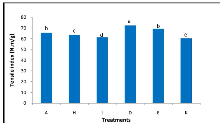
Fig. 4. The effects of CMC and Alum on tensile index
