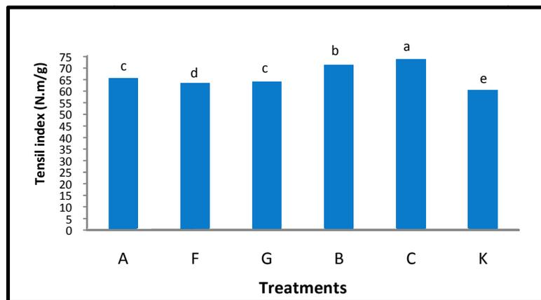
Fig. 2. The effects treatment CMC and surfactant on tensile index
