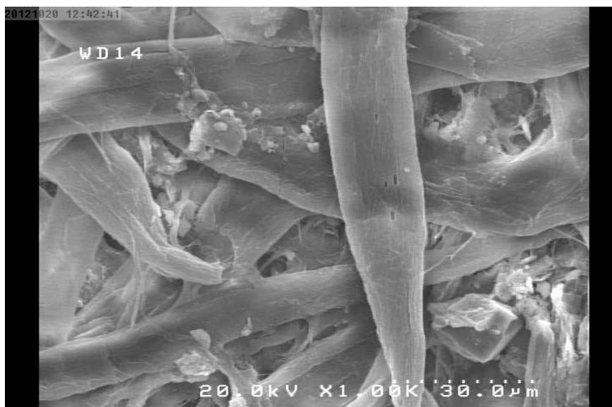
Figure 2. SEM image of talc containing CPAM in the deinked paper
