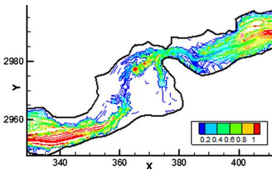
Fig. 5. Map of the flow stream lines coloured by velocity (km/h) in the Gheshm strait after 408h.
