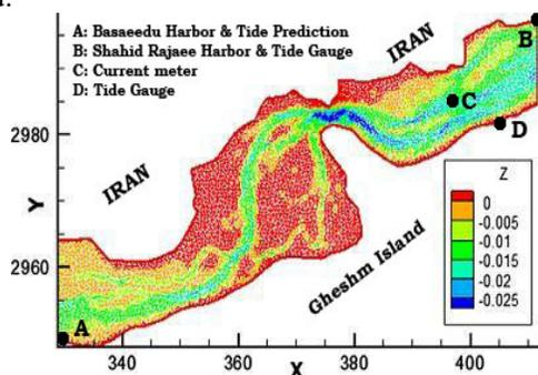
Fig. 1. 2D colored plane mesh of discrete geometrical model (km) and positions of Current meter and tide gauge.
