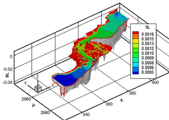
Fig. 4. Colour Coded map of the water level alteration (km) related to mean sea level in the Gheshm strait after 408h.
