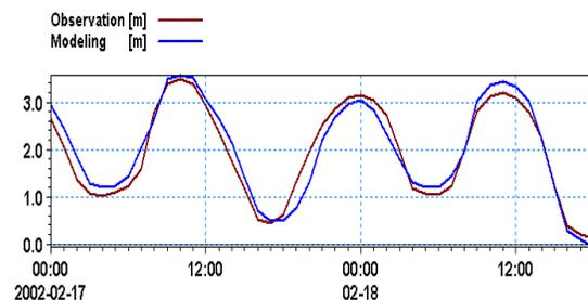
Fig. 2. Comparison of water level with measured values at the kaveh harbor.
