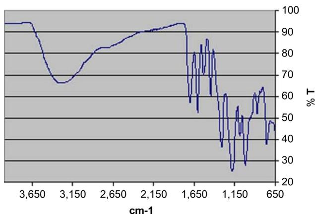
Attractive band in area of 1,325–1,448  $\text{cm}^{-1}$  relates to the bending vibration of methyl group. Attractive band in area of 1,718.09  $\text{cm}^{-1}$  relates to ester carbonyl group. Tensile band (C–O) appears in the area of 1,033–1,203  $\text{cm}^{-1}$ . Resulted spectrum is similar to one presented by Turley *et al.* (1990). Lee and Lan (2006) observed OH group in area of 1,330–1,420  $\text{cm}^{-1}$ .
