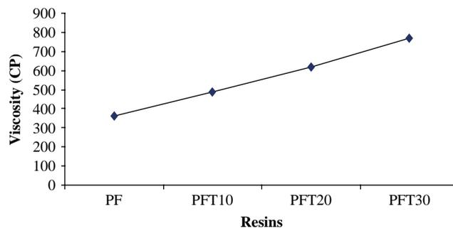
of reaction between tannin and formaldehyde, and it then reduces because of the reduced reaction rate. Tannin affects the viscosity of PF resin significantly. When tannin comes into PF resin system viscosity increases from 360 centi pose to 480, 610 and 760 centi pose, respectively, (Figure 7).
