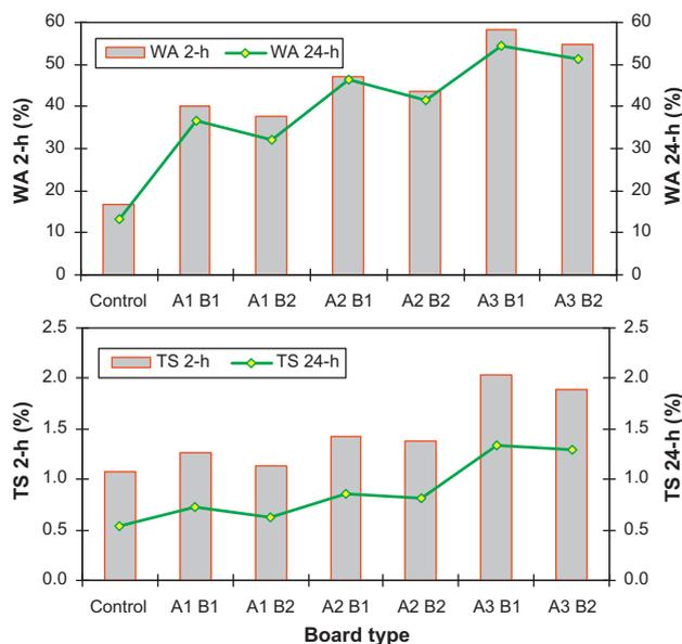
Fig. 3. Effects of RNP and  $\text{CaCl}_2$  contents on the WA and TS of boards.
