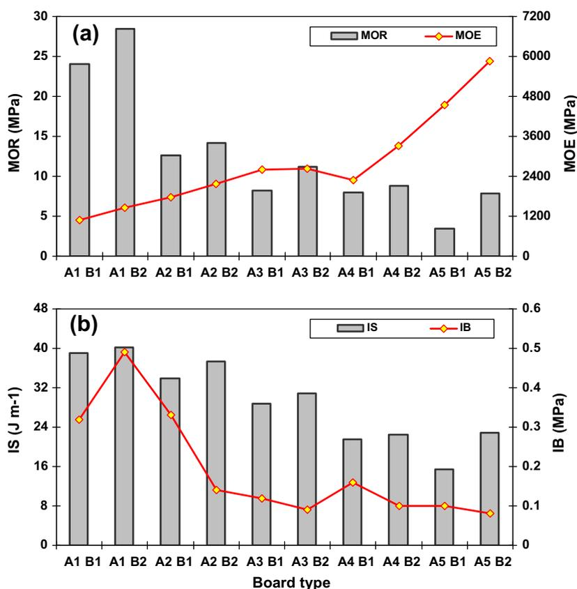
Fig. 1. Mechanical properties of various board types.
