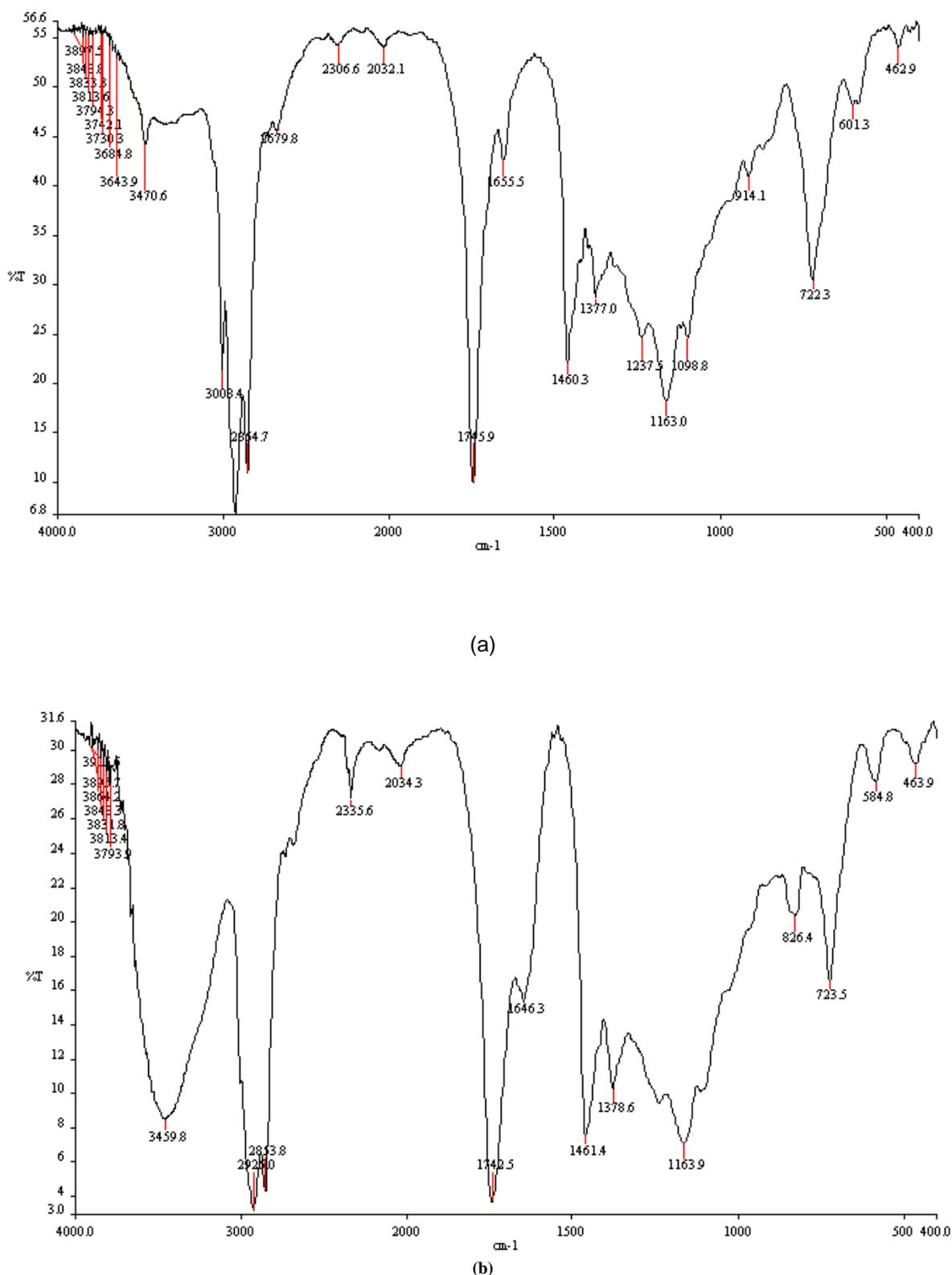
Figure 3: FTIR spectrum of soybean oil (a), ESO (b) to show functionality available in raw materials and products of the epoxidation.
