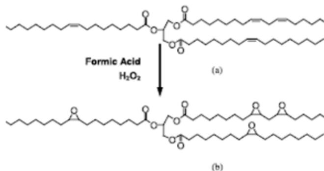
**Figure 2.**production procedure for ESO: (a) triglyceride molecule, (b) epoxidized soybean oil (ESO)
