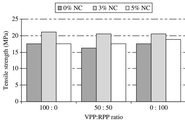
Figure 1. Effects of nanoclay (NC) content and polypropylene type on tensile strength. VPP = virgin polypropylene; RPP = recycled polypropylene.
