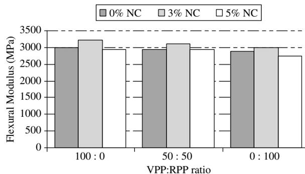
Figure 4. Effects of nanoclay (NC) content and polypropylene type on flexural modulus. VPP = virgin polypropylene; RPP = recycled polypropylene.
