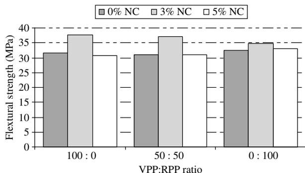
Figure 3. Effects of nanoclay (NC) content and polypropylene type on flexural strength. VPP = virgin polypropylene; RPP = recycled polypropylene.
