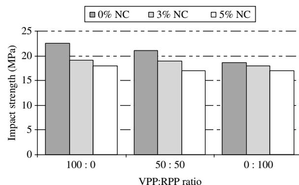
Figure 5. Effects of nanoclay (NC) content and polypropylene type on notched impact strength. VPP = virgin polypropylene; RPP = recycled polypropylene.
