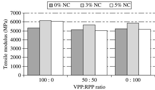
Figure 2. Effects of nanoclay (NC) content and polypropylene type on tensile modulus. VPP = virgin polypropylene; RPP = recycled polypropylene.
