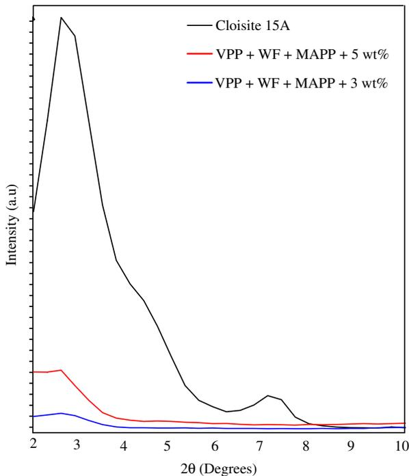
Figure 6. X-ray diffraction patterns of clay (cloisite 15A) and its polypropylene composites with wood flour. VPP = virgin polypropylene; WF = wood flour; MAPP = maleic anhydride grafted polypropylene.
