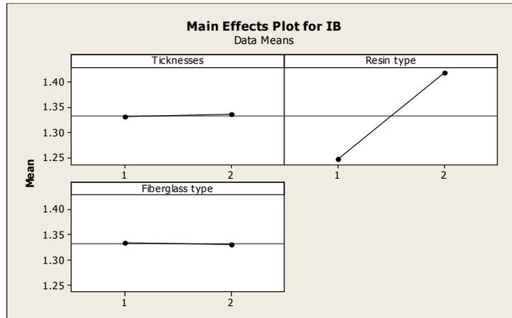
Fig. 5. Effect of different treatments on Sandwich panel, flatwise tensile strength
