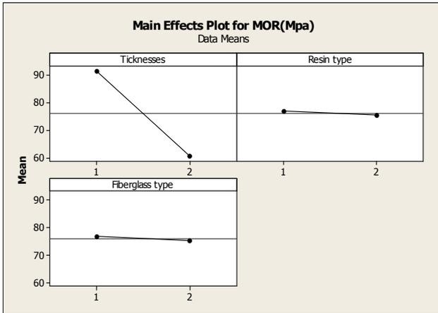
Fig. 2. Effect of different treatments On bending strength
