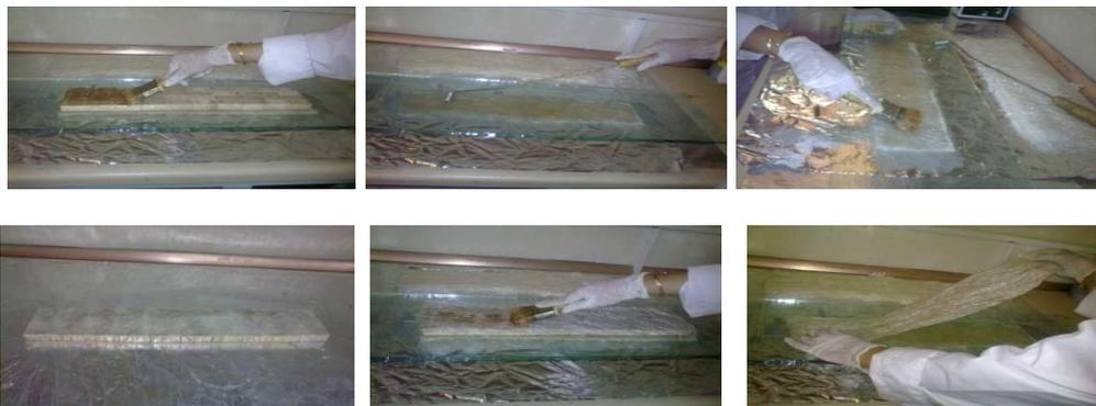
Fig. 1. some stages of sandwich panel production (right to left)
