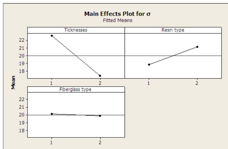
Fig. 4. Effect of experimental factors on sandwich panel, compressive strength
