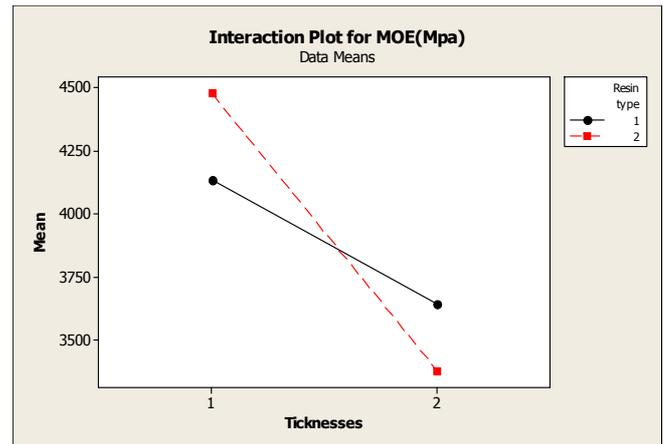
Fig. 3. Interaction effect between the resin and thickness on bending strength
