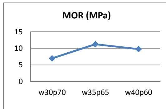
Fig. 2: MOR of Wood flour/ recycled polypropylene composites.
