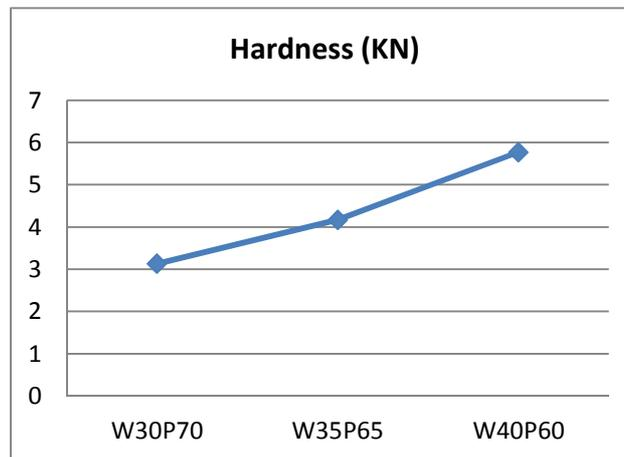
Fig. 3: Hardness of Wood flour/recycled polypropylene composites.
