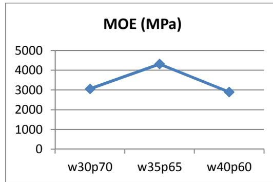
Fig. 1: MOE of Wood flour/ recycled polypropylene composites.
