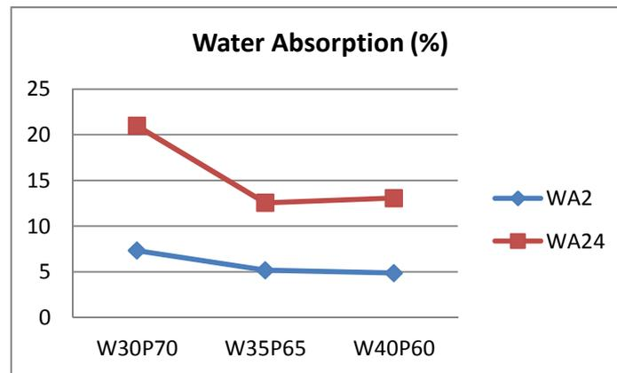
Fig. 4: Water absorption after 2 and 24 hours
